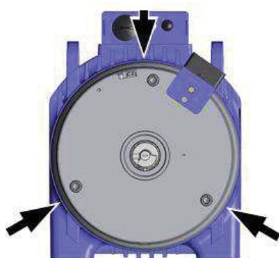
Figure 8-2-1-01 - Air gap measurement position
