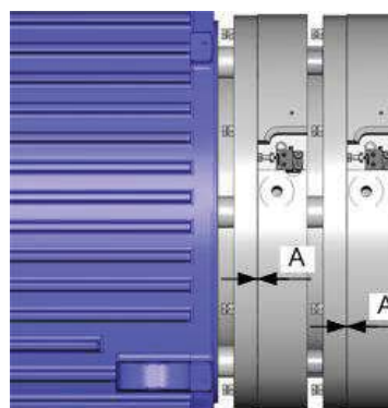
Figure 8-2-1-02 - Air gap measurement
